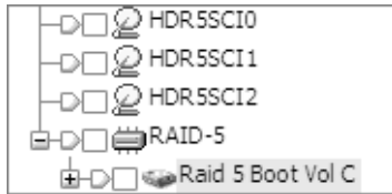
FIGURE 6.8 Three physical devices from a hardware RAID 5 configured and mounted as a logical RAID 5 within EnCase. Note the “RAID” icon, which is a gray box with six protruding red lines.
